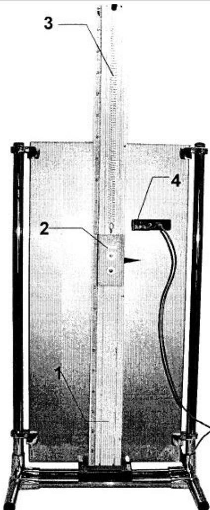
1. Assemble the laboratory unit by fixing the end of one of the springs to the top of the support structure, and attaching the carriage without a load to the other end. Place the optical sensor in the path of the carriage plate.
